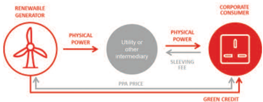
Figure 7: Back-to-back PPA structure diagram
